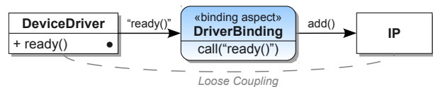
Figure 6: The principle of loose coupling. A binding aspect establishes a relation between two otherwise unrelated modules. The invocation of ready() is translated to an add() call, which registers the DeviceDriver at the IP stack.
